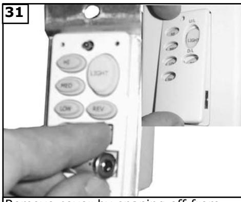
31 Remove cover by snapping off from top or bottom. Install 12V battery into wall remote. Duracell MN21 / Eveready A23 / GP 23A all 12V.
